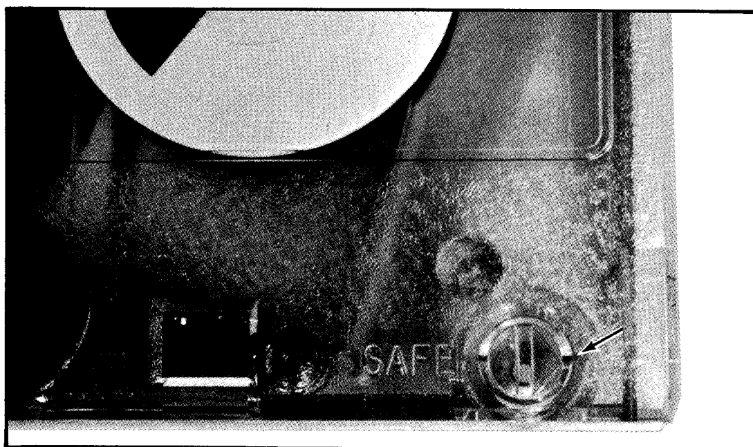
Figure 12. Tape cartridge safety lock off (read-write position)
